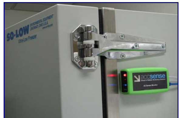
Accsense Monitor on Ultralow Freezer
