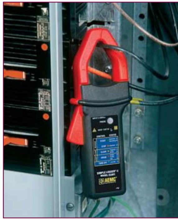
Easily log current in power panels.
