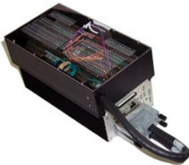
DAQ750 shown with cover removed
