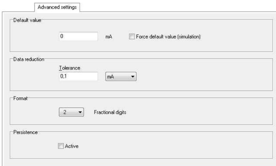
**Default value:** This is used in the event of a input or output failure (refer also to [status monitor](#) ). The settings depend on channel type. For example, digital inputs have only the options *Off* and *On*.
