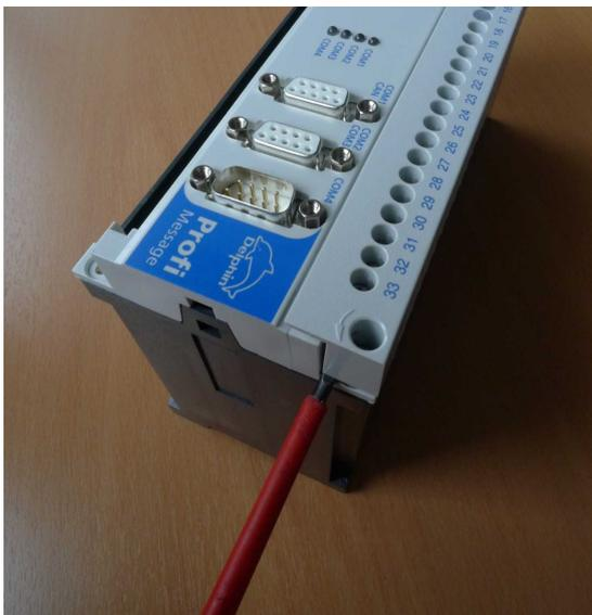
5. Use a screwdriver to lightly press the two retaining lugs at the housing sides and lever towards the front.
