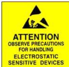
Electronic components are sensitive to ESD (**E**lectro-**S**tatic **D**ischarge). Therefore, discharge any electrostatic energy before opening the device for I/O module or memory card installation/replacement. We recommend wearing a wrist band (static discharge wrist band) and to carry out the work on a conductive surface.
