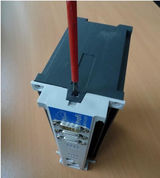
6. Remove the memory card from its slot using long-nose pliers or a similar tool.
