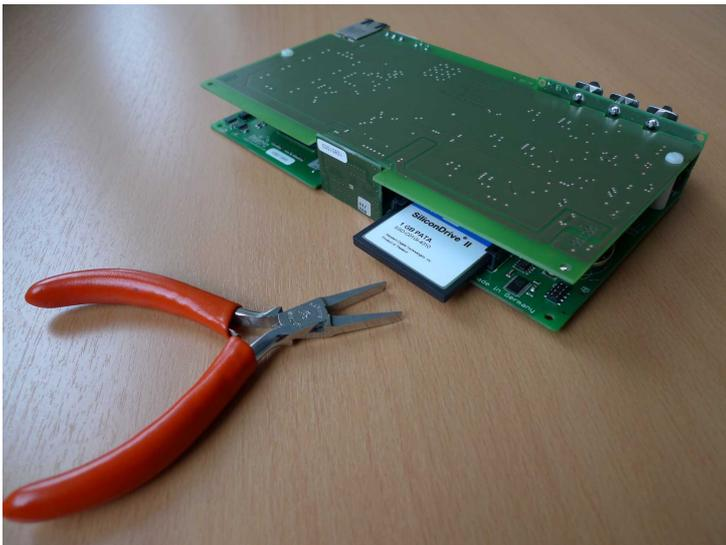
7. Push in the new memory card, with its "handle" pointing towards the board, until it stops. Use only gentle pressure and do not force. The card fits in one direction only.
