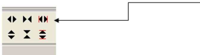
The symbol on the upper right is available only for offline batch processes. It enables portrayal of the entire recorder file. The batch process can then be visualized as a whole.
