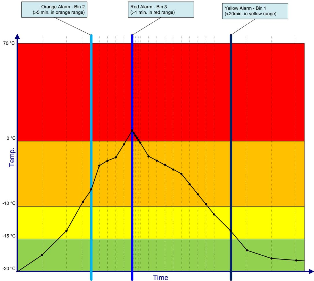
**Fig. 2.2: Frozen example, time vs. temperature view**
