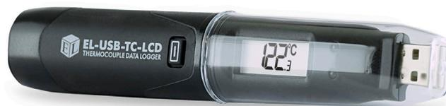
This standalone data logger measures and stores more than 32,000 temperature readings from a J, K or T-type thermocouple at a resolution of 0.5°C (1°F). It comes supplied with a K-type thermocouple capable of measuring from 0 to 200°C (32 to 392°F).
