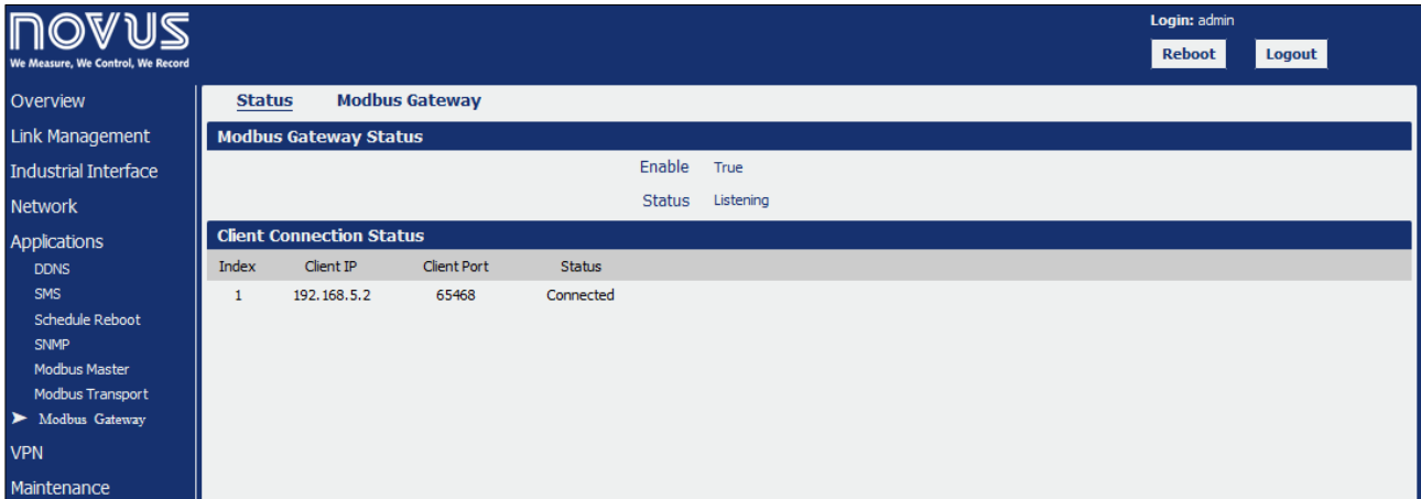
Figure 160 – Modbus Gateway application
